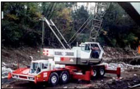
Igel purchases Bucyrus Erie 65-C high tensile strength boom cranes. Lighter, stronger metal allows for greater load-lifting capacity.
